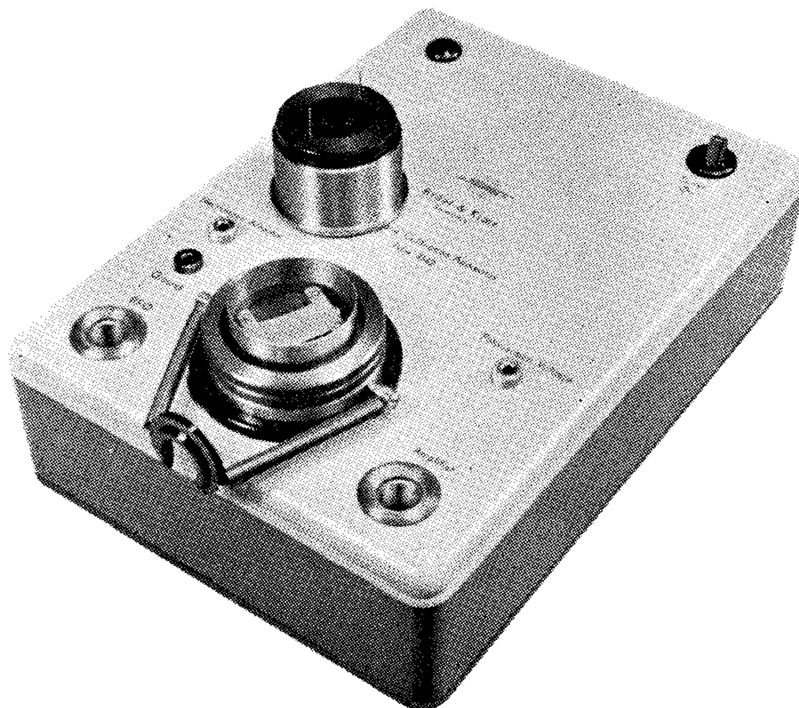
Fig. 17. Photograph of the Thermophone made for these tests. A thin nickel foil was used instead of the usual gold foil.
